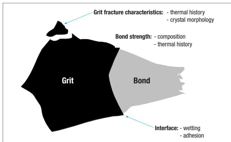
Fig 2 Parameters for optimising the vDD system
