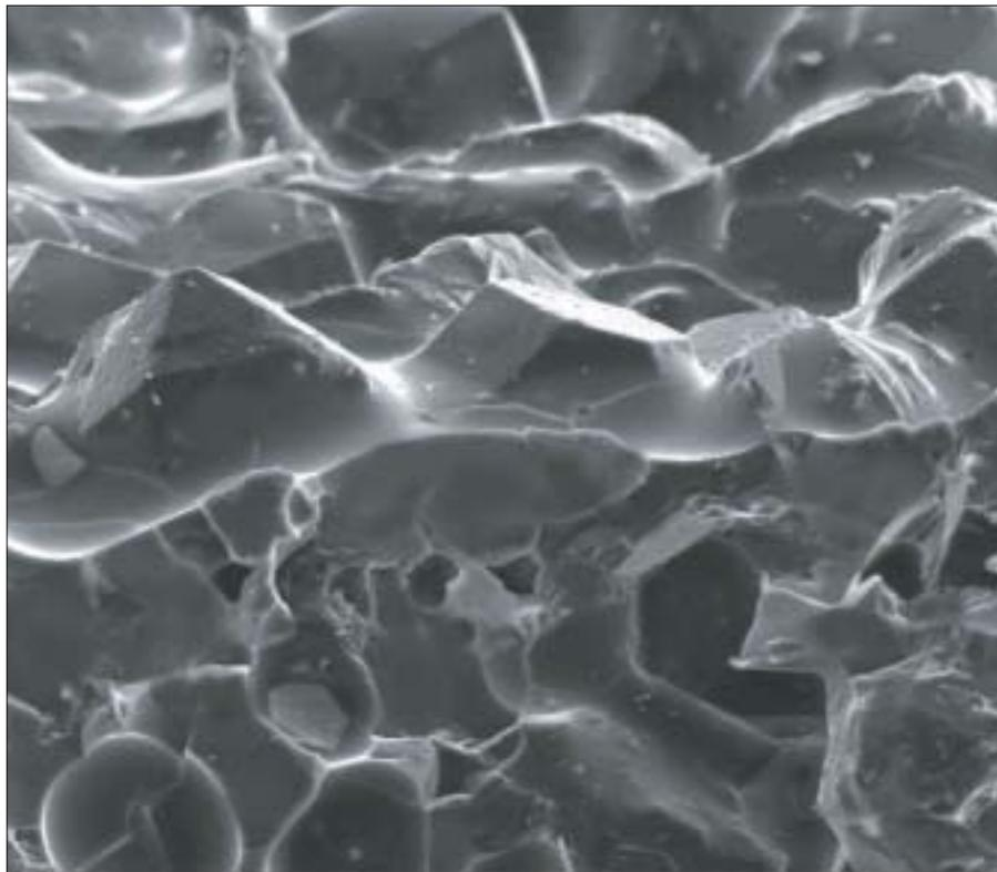
Fig 3 SEM of a vDD structure (200x). Structure with spherical pores (bottom half of the image) and a surface with optimally wetted grains and at the same time a high grit protrusion (top half of the image)
